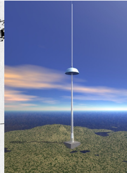
Present version of entire CODAR antenna initiated at NOAA under Dr. D.E. Barrick in 1972
